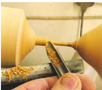
▲ Pic.9 Work the stem down in sections, about an inch at a time; when you have finished one part move onto the next, but don't go back to the top as you will break it
